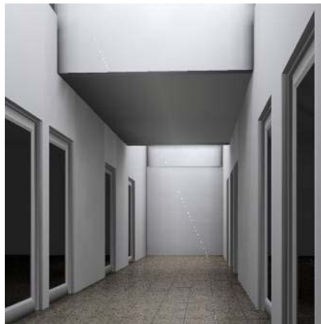
Revit radiosity view showing daylight only.
