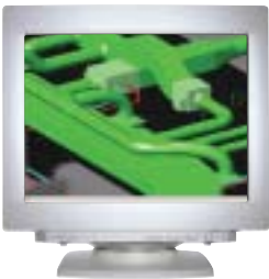
A 3D representation of HVAC and electrical systems allowed Flack + Kurtz engineers to detect interferences before construction.
