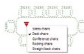
Visibility Control Use a drop-down menu to select variations on block geometry.
